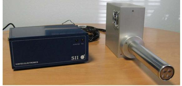
Figure 1. The Vortex- $ME^{TM}$  multi-element detector system. Left to right: PS box, cable, SDD package.
