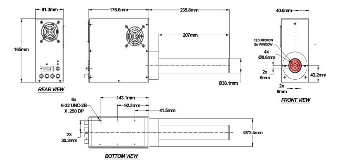
Figure 4. Vortex-ME<sup>TM</sup> SDD package with external dimensions (in mm).
