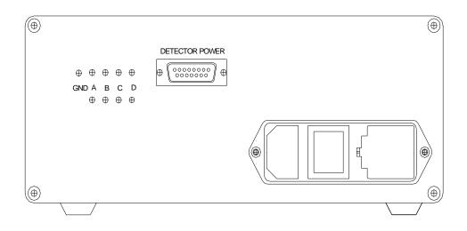
Figure 6. Back panel of PS electronics box.
